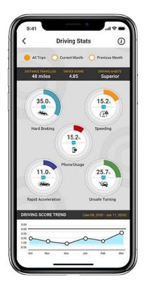
Telematics devices installed in vehicles or smartphone apps collect data on driving behaviour, including factors like speed, acceleration, braking, and cornering. This data is then transmitted to insurance companies, allowing them to analyse driving patterns and assess risk more accurately.
