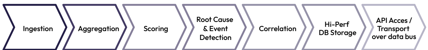
Figure 2: Data pipeline stages for finding customer experience score
